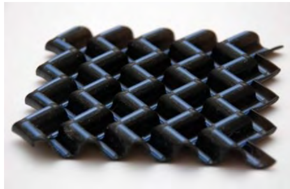
Figure 6. The first replication of the geometric model. A rubber 3D-print with plastic ligaments.
