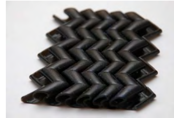
Figure 8. Second replication of the geometric model using rubber only and increased condensing of the form.
