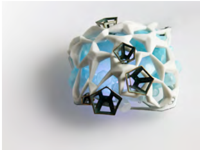
Figure 1. The Geotronic Brooch contains a programmable colour LED which is set to beat like a human heart.
