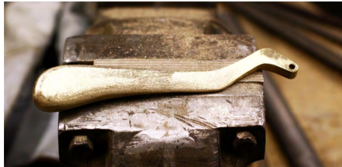
Figure 9. Filing and refining final tool.
