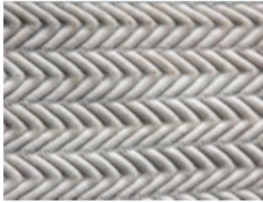
Figure 5. Close-up of knitted auxetic fabric.
