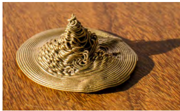
Figure 3, 45° cone, 'failed' print.
