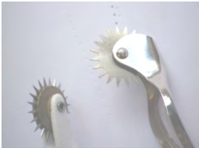
Figure 2. Existing Plastic handle Tracing Wheels. The tool on the left has burs left by the plastic molding processes that are sharp in the palm of the hand. The tool on the right has a pressed metal wheel with blunt serrated points.
