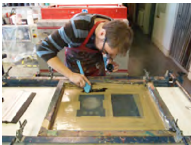
Figure 4. Using a traditional screen printing technique to experiment with the emerging technology of conductive inks.
