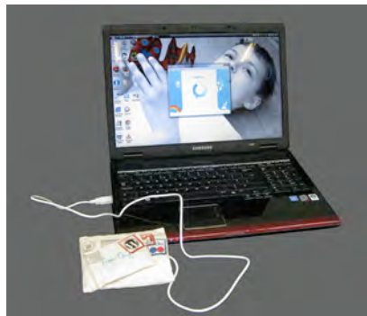
Figure 7. Pigeon Post Project; soft textile tags connecting to Skype via RFID tag and reader.
