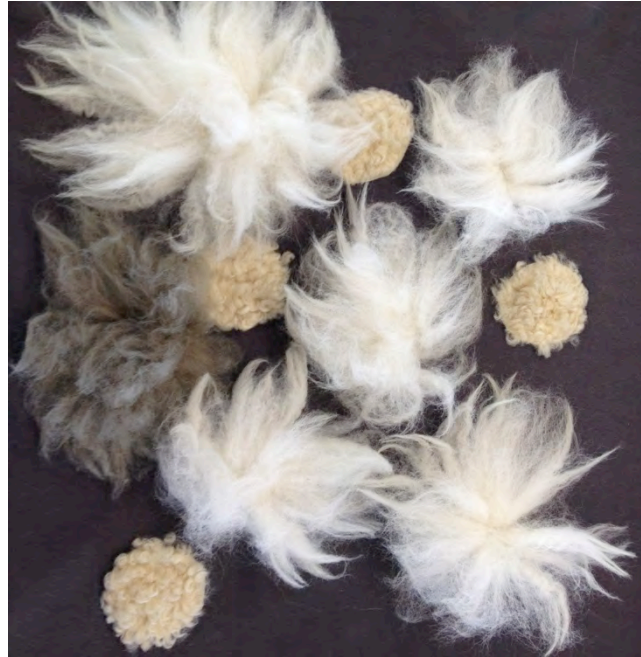
Figure 4. Sheepskin shapes bonded to adhesive prior to trimming.
