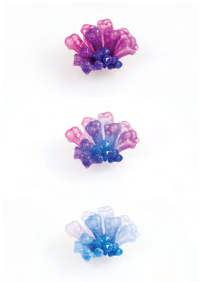
Figure 3. A temperature induced colour change cycle (low to high) from magenta to blue in thermochromic silicone samples for the Cocoon Earring series.
