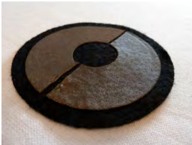
Figure 8. A conductive fabric pad on the table cloth connects the saucer to a microcontroller on the table. The semi-circular grey sections match with the underside of the saucer. Using soft conductive fabric allows the rigid ceramic to make good electrical contact.
