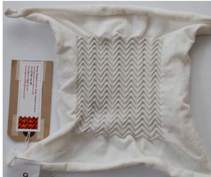
Figure 3. Weft-knitted auxetic structure shown in placement on plain knitted fabric.
