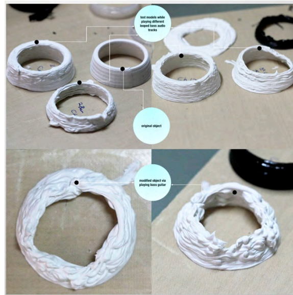
Figure 3: Resulting Objects - The comparison of initial test tube model, modified with audio loops and live guitar session.
