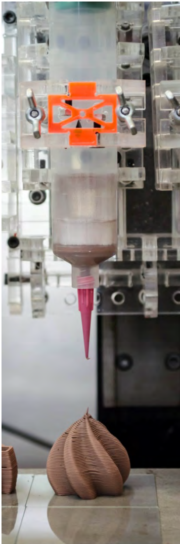
Figure 1, Machine setup, depositing 'seashell' build in bronze
