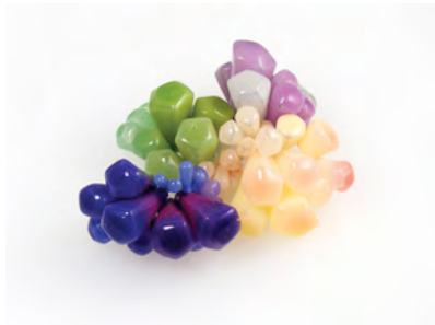
Figure 4. Below is an example of the colour range achievable in combining thermochromic Leuco Dyes with Silicone
