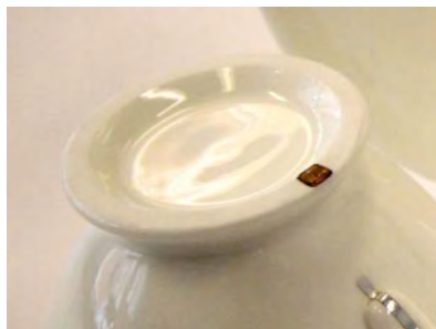
Figure 6. The protrusion on the cup is made of copper which is able to connect the switches on the saucer surface. This is shaped to sit on the inside rim of the saucer surface.
