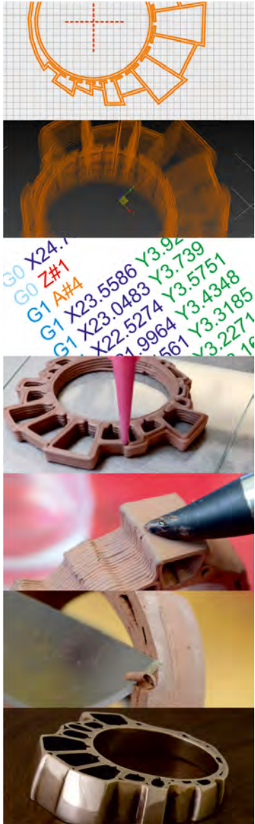
Figure 2, Process film strip, from design to product, in BronzClay
