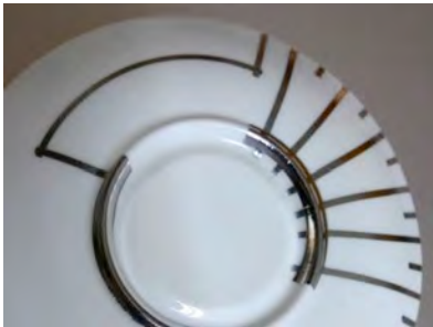
Figure 7. The underside of the saucer has two semi-circular contacts on its central rim that lead to either of the two sets of radial switch contacts on its surface.
