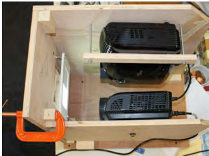
Figure 2. The 4 th Wall Viewer prototype, using synchronized HD projectors focused on a rear projection viewer.
