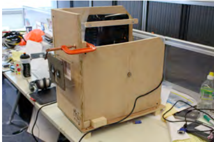
Figure 1. The 4 th Wall Viewer prototype, using synchronized HD projectors.
